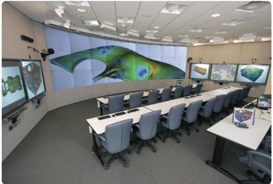
*The need for such an ambitious assembly at the Sandia National Laboratories' Interactive Design Center (IDC) in Livermore, CA was driven in large part by the video rendering firepower that Sandia has available for it. With each node connected to one of the 27 projectors, there's a one-to-one relationship between computer and projector.*
