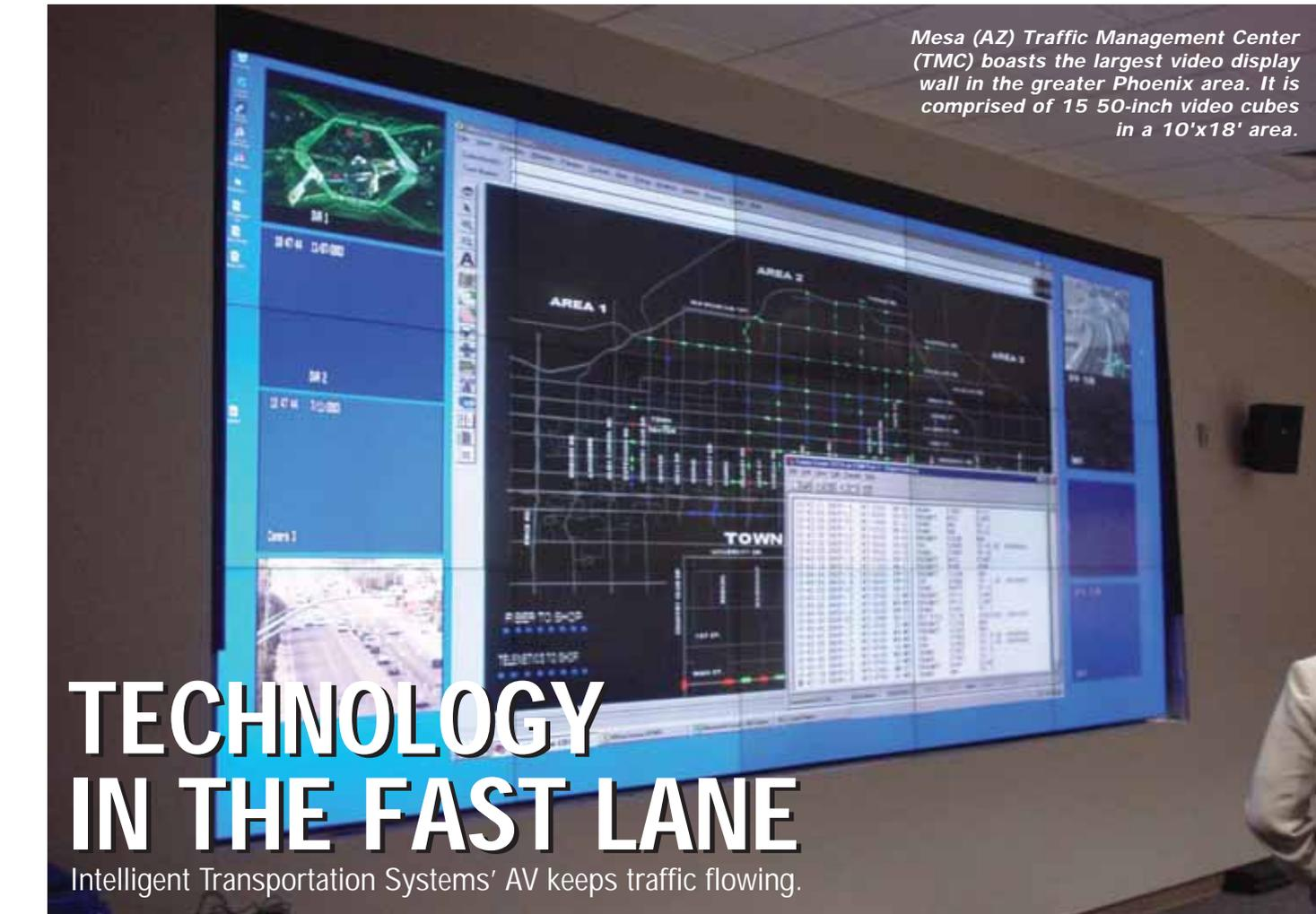
Mesa (AZ) Traffic Management Center (TMC) boasts the largest video display wall in the greater Phoenix area. It is comprised of 15 50-inch video cubes in a 10'x18' area.
